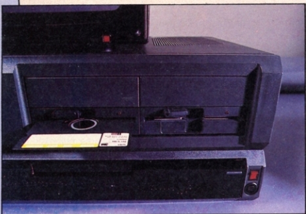
Advance storage: 360K floppy disk drives, with latches to keep the disks in place, for the more expensive machine. For the cheaper machine, a DIN-plug cassette port.
